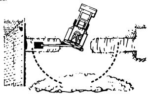
Position the unit forward with the lift and crowd levers so the two trenches can be connected. Pile the spoil on the opposite side of the trench.
